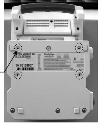
2. Ensure four (4) standoffs on Sub Plate are facing away from the monitor (see below), and fasten Sub Plate to rear of monitor with four (4) #6-32 x 3" PHMS as shown below.
