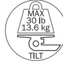
Maximum weight for mounting plate with tilt function.
