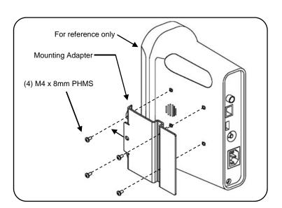
2. Pull Spring Plunger at the front of the Mounting Plate and slide device laterally into the Mounting Plate until the Plunger snaps into the clearance hole at the front of the Mounting Adapter. Tighten the (4) Nylon Locking Screws located on bottom of the Mounting Plate.
