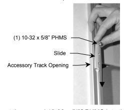
4. Insert the second 10-32 x 5/8" PHMS into the Slide and tighten both to secure Channel in position.
