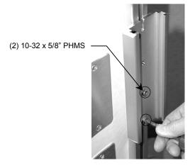
3. Insert the second (top) Slide into the Accessory Track opening and slide behind the Channel so the top screw enters the slot at the top of the Channel.
