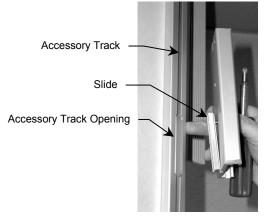
2. Position the Channel and tighten the (2) 10-32 x 5/8" PHMS to secure the Slide in the Accessory Track.
