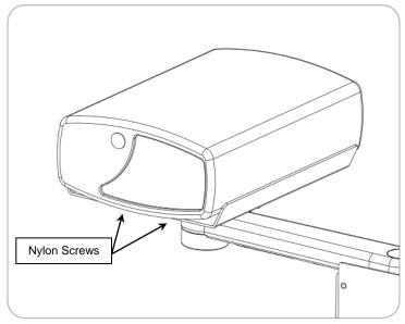
2. Tighten the (2) Nylon screws located towards the front of the mounting plate to secure.
