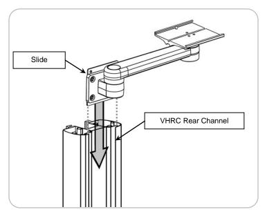
2. While supporting the bottom of the arm, guide the slide into the top of the VHRC rear channel and move arm to required mounting position.
