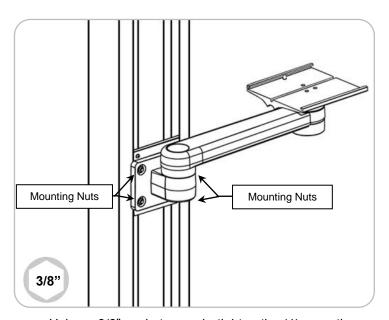
4. Using a 3/8" socket wrench, tighten the (4) mounting nuts to secure position of the arm. Re-install top cover and screws that were removed in Step 1.
