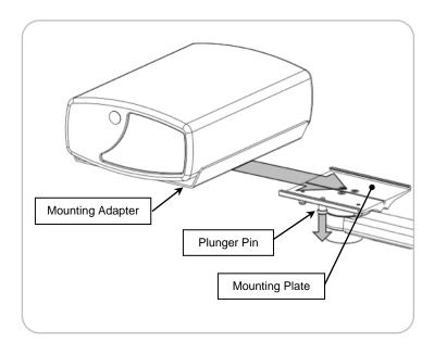
1. Pull the plunger pin at the front of the mounting plate. Slide the mounting adapter into the mounting plate until the plunger pin snaps into the clearance hole in the adapter.
