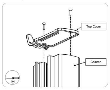
Using a Phillips screwdriver, remove the (2) mounting screws and top cover from the VHRS column. Set these items aside.
