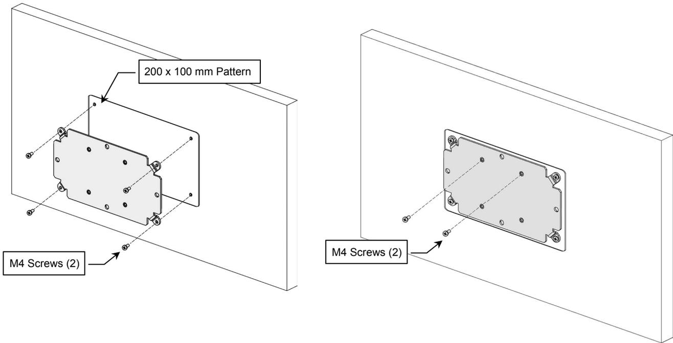
3. Lift display onto VESA Mounting Plate by guiding M4 screws into slots in top of Plate (below left). Thread two (2) M4 screws into lower mounting holes (below right). Tighten all screws.
