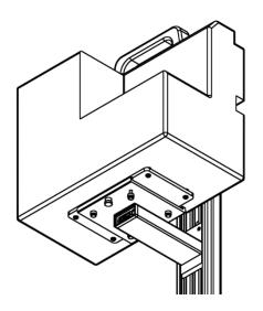
The purpose of this manual is to describe general installation of DSC-8430 Flush Mount to Channel. This manual should be used in conjunction with any instrument-specific installation guides. Please read this manual and all instrument-specific installation material before installing or using this product.
