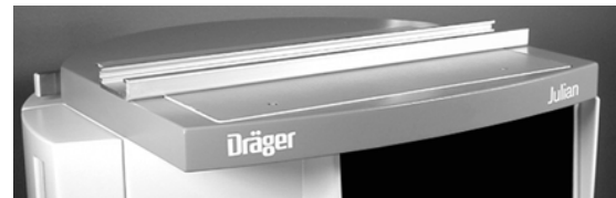
View of installed Spacer Bars. Bars have double sided VHB tape to secure to Julian top shelf.
