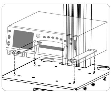
2. Lower the Corometrics/GE250 onto the tray aligning (4) locating pins on the tray slide with (4) corresponding locating holes on the mounting rails.
