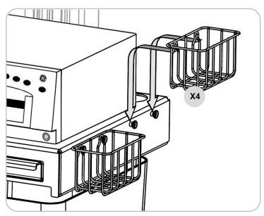
**3.** Install (4) utility baskets by sliding them over the mounting buttons and pressing down.
