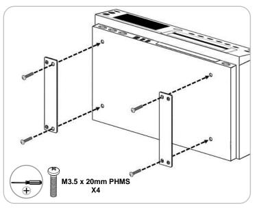
1. Secure the (2) adapter rails with (2) M3.5mm x 20mm PHMS per rail. The locating hole on each rail must be positioned inward.
