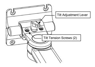
**Installation Note:** The Tilt Adjustment Lever is a multi-position clamping lever that operates by lifting, rotating, and releasing the handle.
