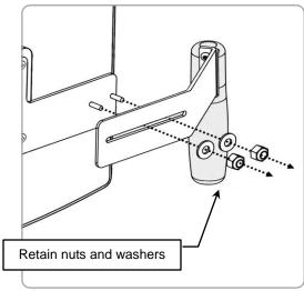
2 Install the holster onto the center plate studs using the 10-32 nuts and washers. Leave the nuts loose so holster can slide in/out. Adjust the spacing between the display and holster, and then tighten the 10-32 nuts to secure the holster. Place barcode scanner into the holster, route cables as needed.
