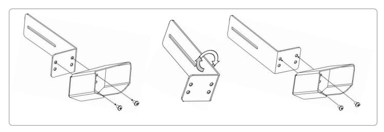
1 Remove the handle from the center plate located on the back of the display by loosening the (2) 10-32 nuts with a 3/8" (10mm) wrench. Keep the flat washers and nuts.
