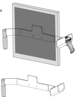
**Installation Note:** The handle/ holster assembly is designed to mount directly to a flat panel display with a 75mm x 75mm VESA mounting pattern on the rear. Displays with a 100mm x 100mm mounting pattern require attachment of GCX P/N FLP-0002-17 (*Mounting Kit for 75/100m VESA Compatible Flat Panel Displays*). The handle and holster are adjustable to fit typical flat panel displays from 11.5" [29 cm] to 18.5" [47 cm] wide (not diagonal measurement).
