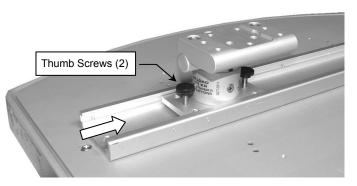
3. Fasten Table Top Mount to Mounting Adapter with one (1) M6 x 12mm FHMS and two (2) M6 x 8mm FHMS as shown.
