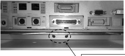
Tighten both (2) 8-32 PHMS when desired positon has been reached.
