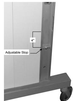
3. Insert Channel Slide (now on rear of CPU) in channel opening and carefully guide CPU to rest against Adjustable Stop.
