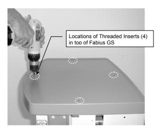
3. Align four (4) mounting holes in Top Plate with corresponding holes in top of machine (drilled in step 2). Fasten Top Plate to machine with four (4) M5 x 30mm Pan Head Machine Screws (PHMS)
